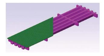
Advanced scripting users can automate the creation of whole bridge spans for beam and slab decks incorporating prestress, design checks and output reports in MS Word.
