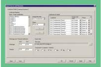
■ Section design checks are carried out in the Deck Designer, from which detailed graphs and reports can be also be output.
