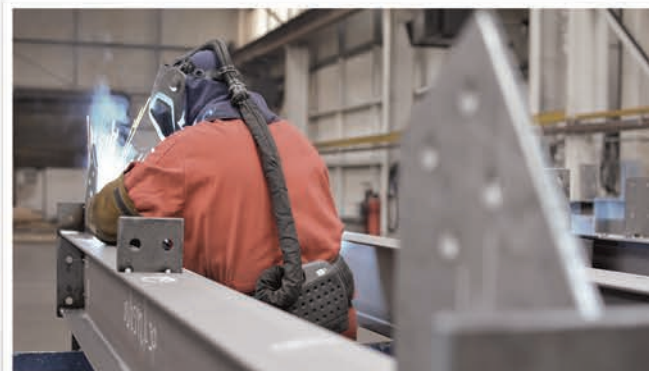
OLD WAY - Manual Tacking and Welding
