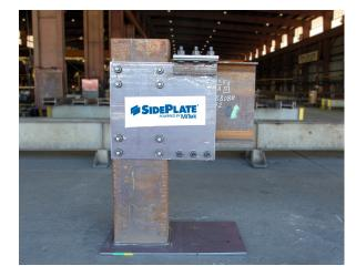
While the All-Bolted Connections solve the issue of a lack of welders and bring options for modularization, there are many other fabrication benefits that the connections bring to the table. SidePlate All-**Bolted eliminates** preheating and distortion control measures that are required when welding. The assembly of the connections is now much faster and easier to lay out and fit-up.
