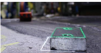
Laser projection showing part placement with Iris SPS.
