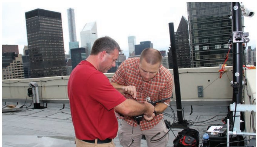
A security engineering officer (right) works on a radio transmitter used to livestream video from security cameras, temporarily installed atop a building in downtown Manhattan during a major event. (U.S. Department of State photo)
