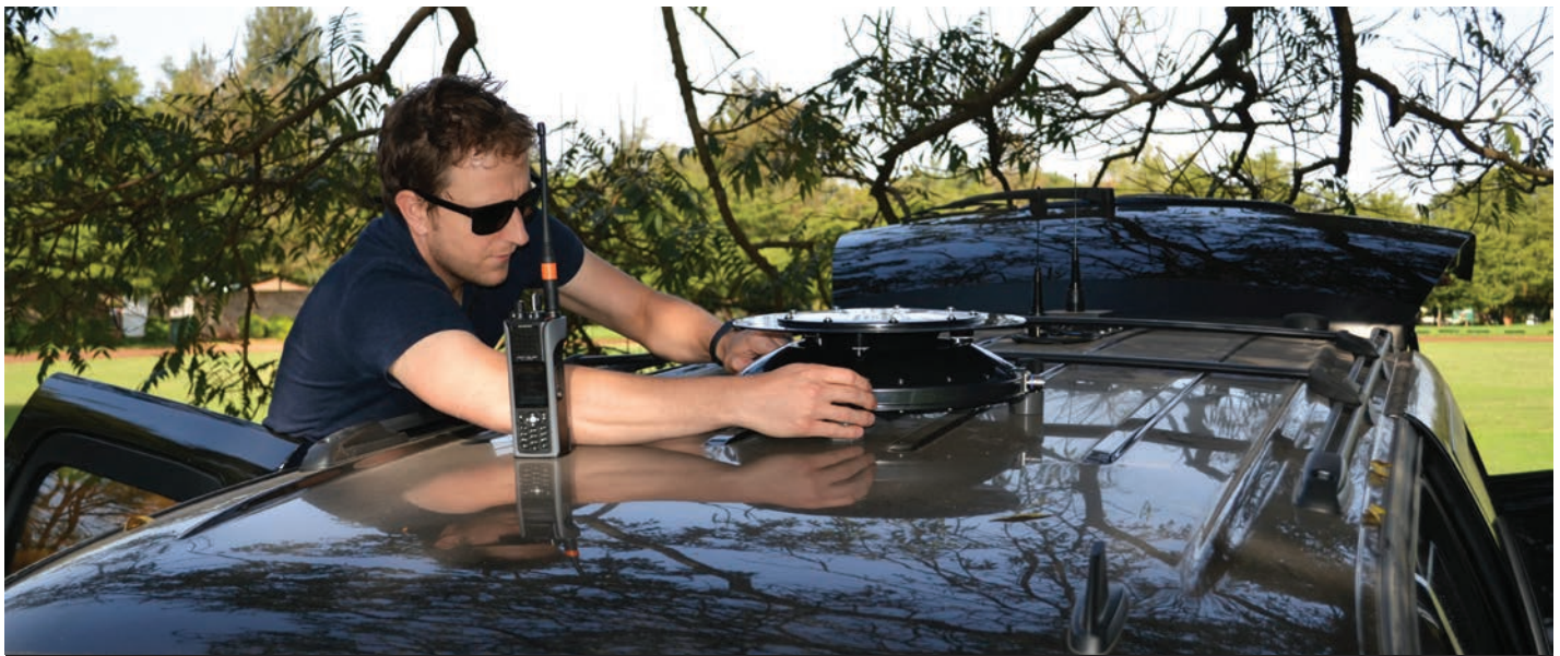
A security engineering officer installs a long-range acoustic device on top of an armored vehicle that transports dignitaries. (U.S. Department of State photo)
